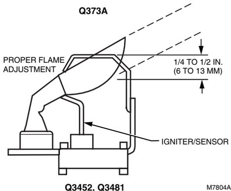
Fig. 17. Igniter-sensor tip must be in pilot flame.
