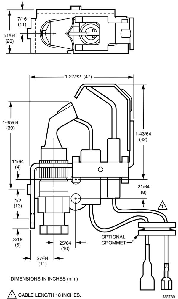
Fig. 10. Q3452 mounting bracket dimensions in in. (mm).
