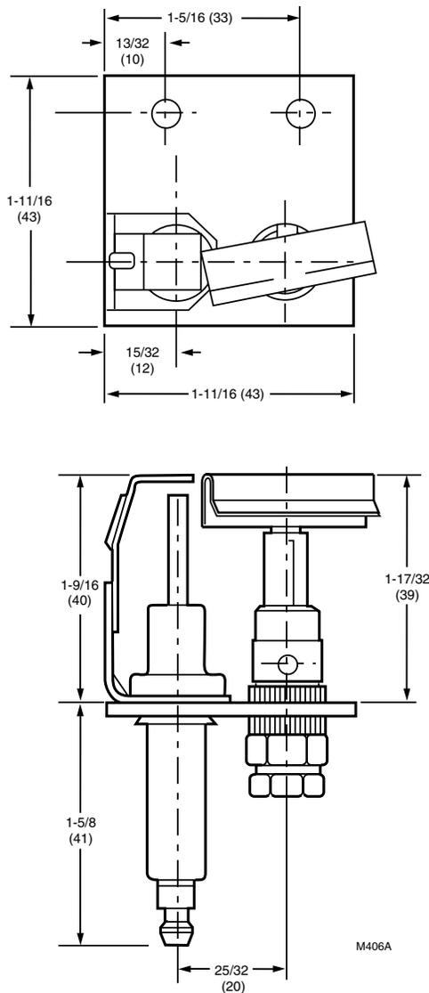
Fig. 9. Q381A mounting bracket dimensions in in. (mm).
