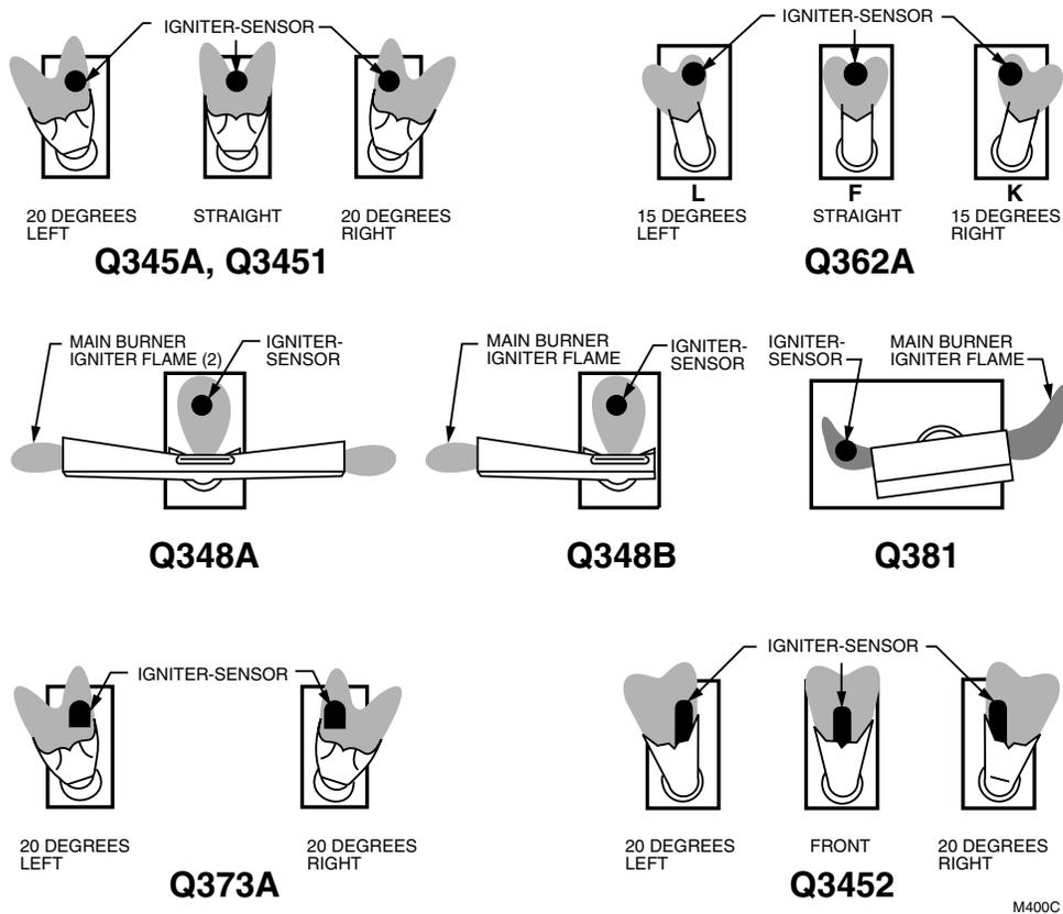
Fig. 12. Pilot burner/igniter-sensor target styles and flame patterns.
